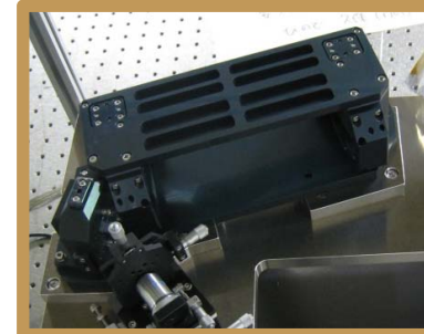
Slitjaw optics: mirror unit & filter unit
