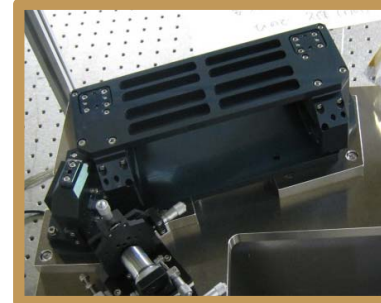
Slitjaw optics: mirror unit & filter unit
