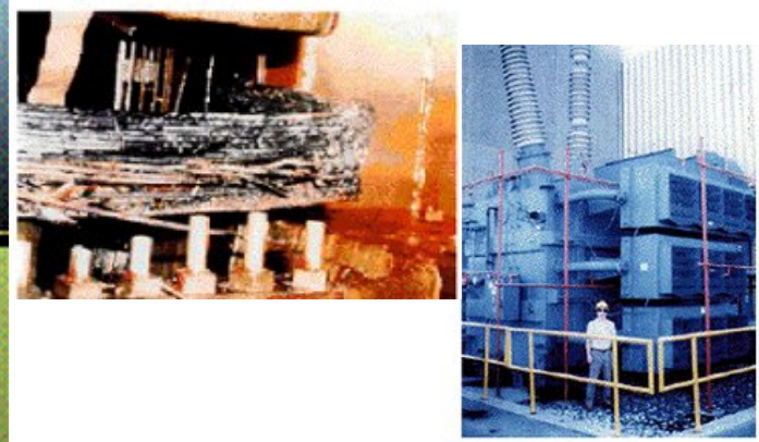
PJM Public Service Step Up Transformer Severe internal damage caused by the space storm of 13 March, 1989
