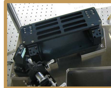
Slitjaw optics: mirror unit & filter unit
